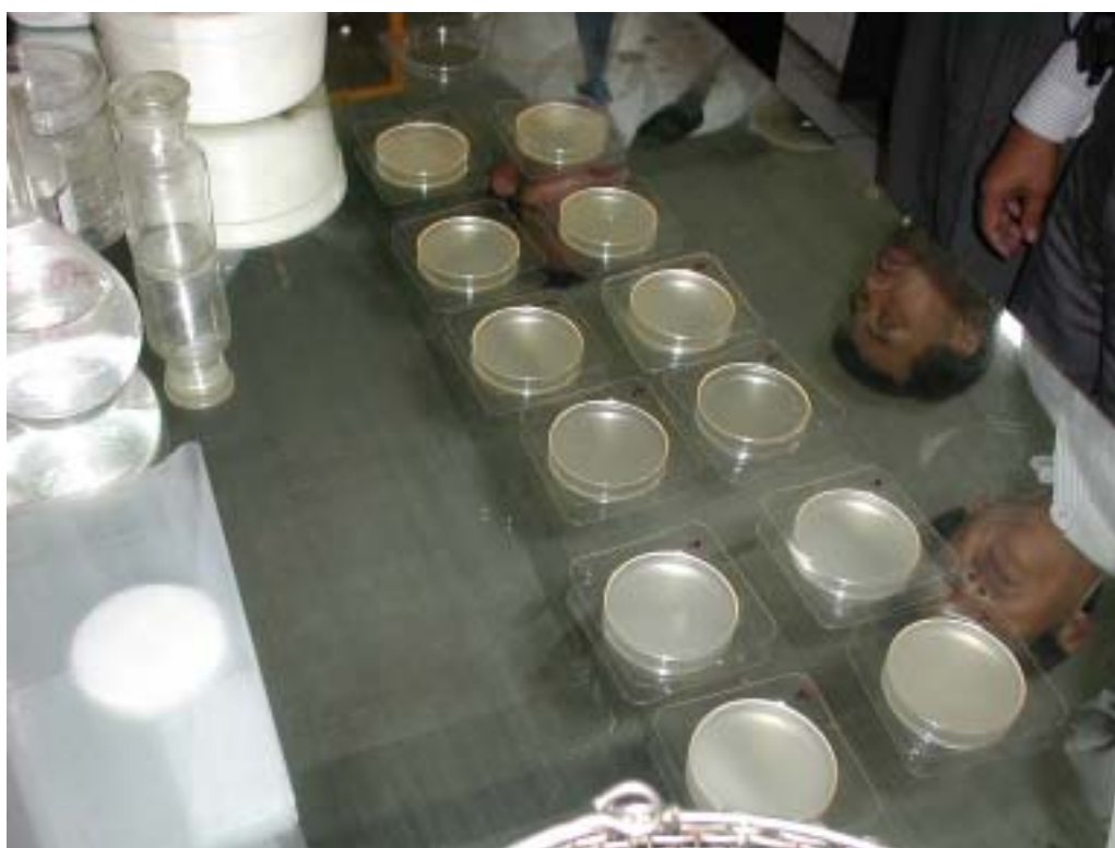
Figure 5 Preparation of hydrogels by radiation crosslinking in Indonesia
