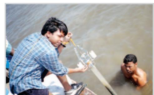
Fig. 2 Sampling of sediment with Kajak corer
