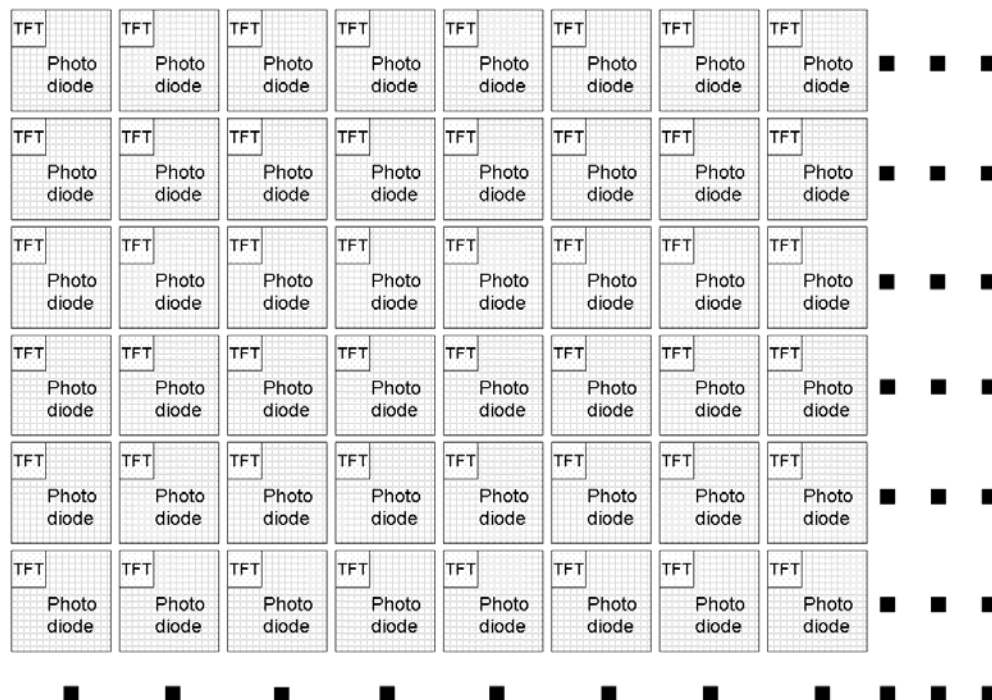
Fig. 7.1: Matrix principle of the arrangement of photo diodes in a digital detector array
