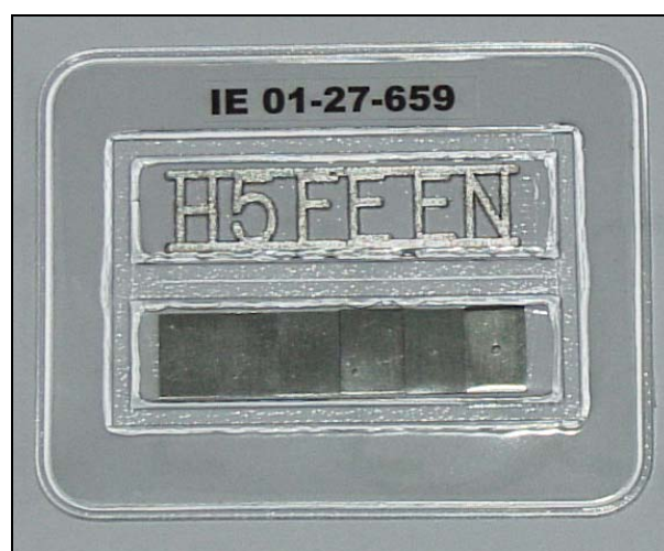
Fig. 4.4: Step hole penetrameter according to EN 462-2 (and ISO 19232-2)
