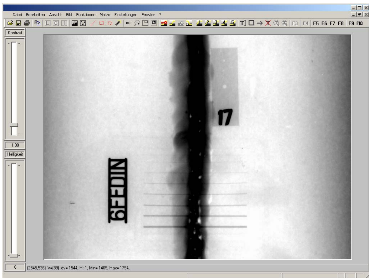
Fig. 8.2: Presentation of an X-ray image together with control panels on the same screen
