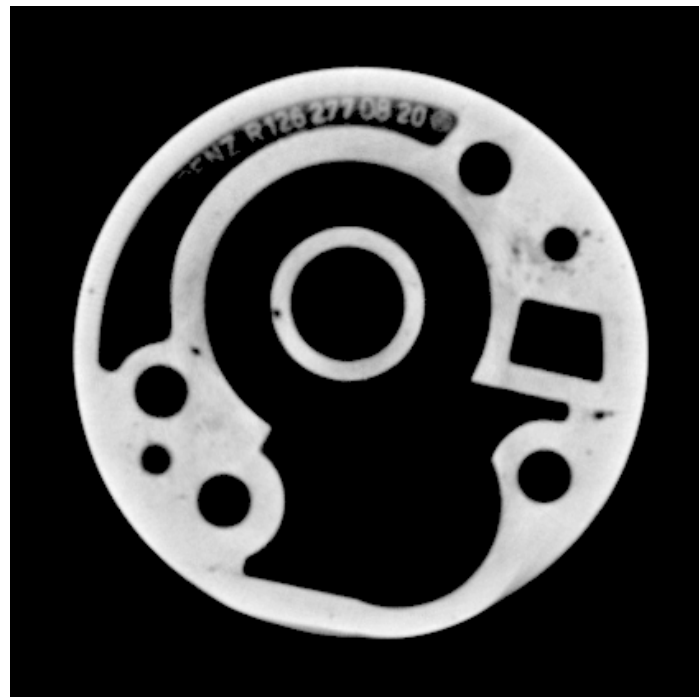
Fig. 16.9: Section through the XY-plane of the tomography of a component
