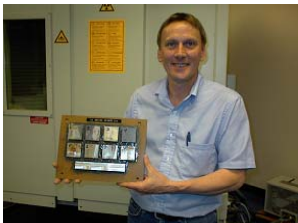
Fig. 13.4: Size of a ASTM E155 plate (reference hardware)
