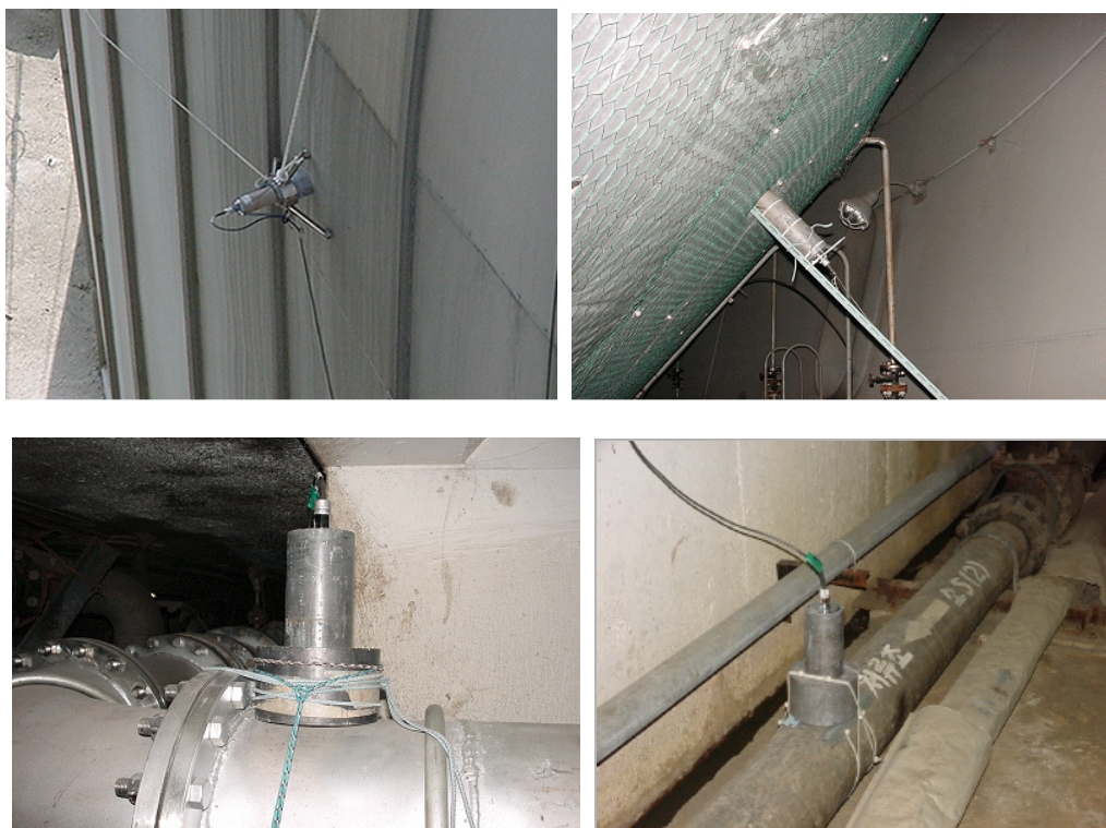
FIG. 105. Some NaI detectors installed around digester
