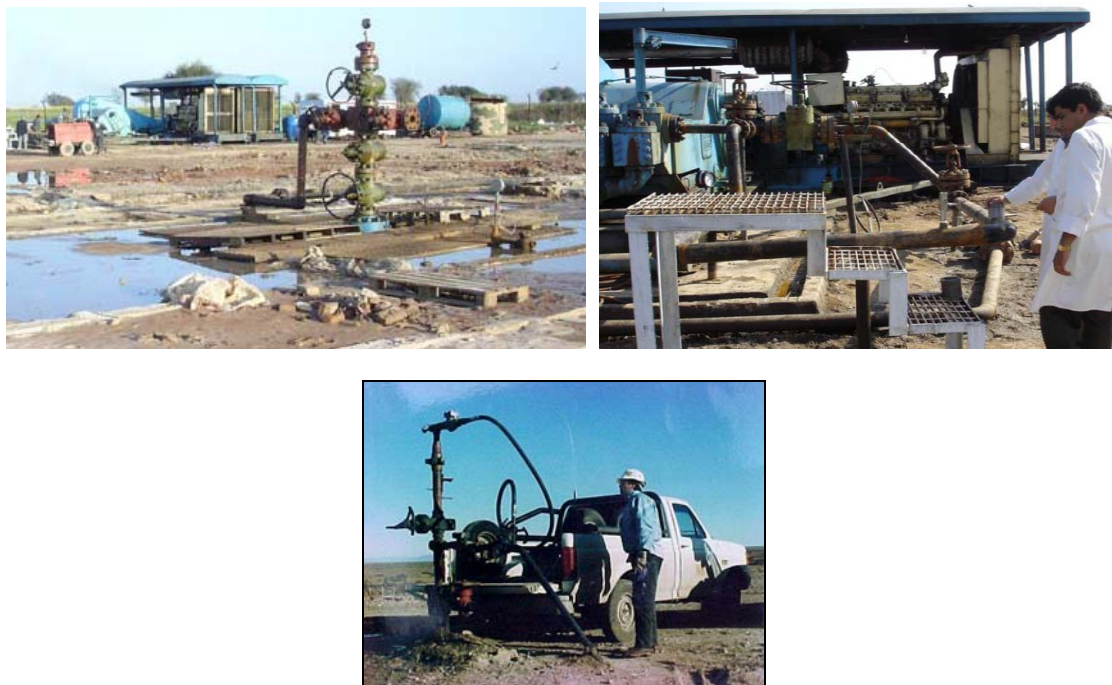
FIG. 113. Tritium injection using bypass technique.
