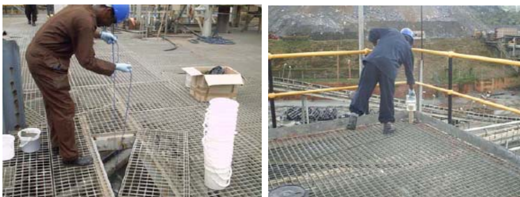
FIG. 71. Taking samples (left) and measuring them with Marineli can on top of NaI detector (left)
