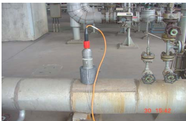
FIG. 18. On-line detection of gamma emitting radiotracer: NaI probe with collimator mounted at the reactor outlet.
