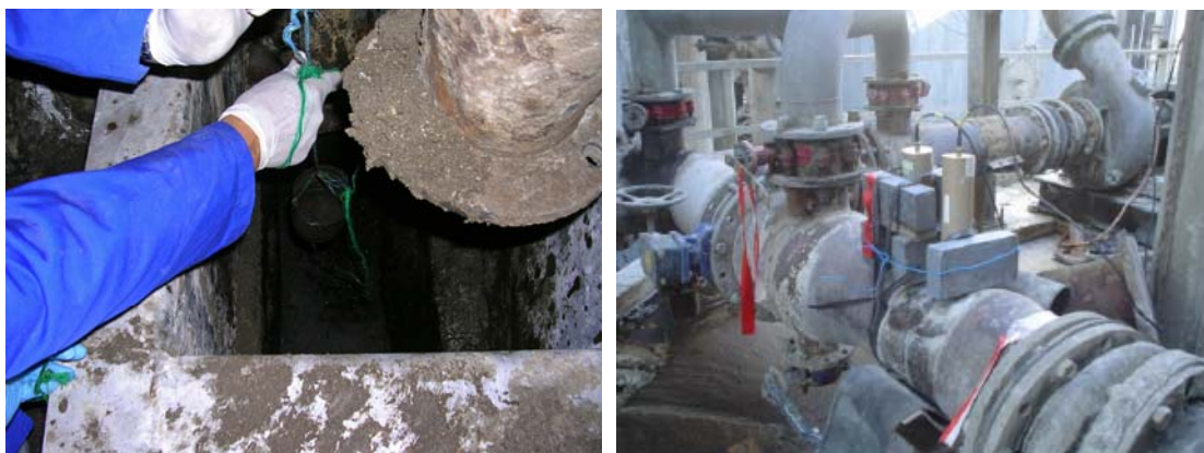
FIG. 68. Injection of the radiotracer at the central unit, and the radiation detector at the outlet of the reactor for online RTD measurement.
