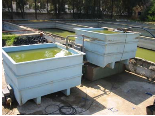
FIG. 137. Pilot scale system of two tanks in series where water moves by gravity
