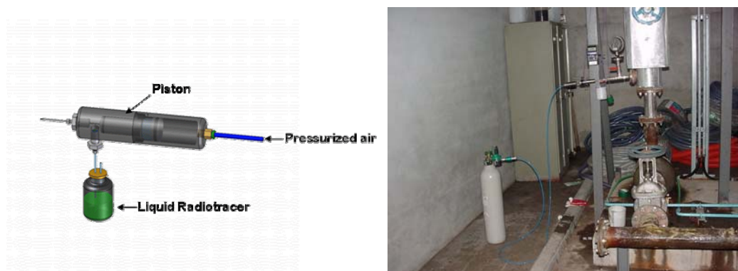
FIG.38. Liquid tracer injector(left shielded syringe, right on site with gas bomb)
