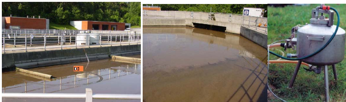
FIG.96. Location of probes: D_2 immersed and D_3 inside detection chamber
