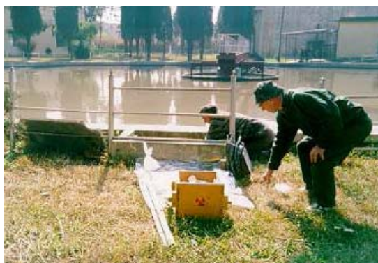
FIG.68. Radiotracer injection in the primary clarifier
