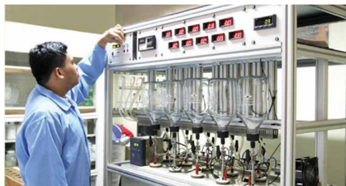
Figure 2. A PNRI researcher using the ultra-low-level tritium enrichment system to determine the age of groundwater samples (Photo c/o DOST-PNRI)
