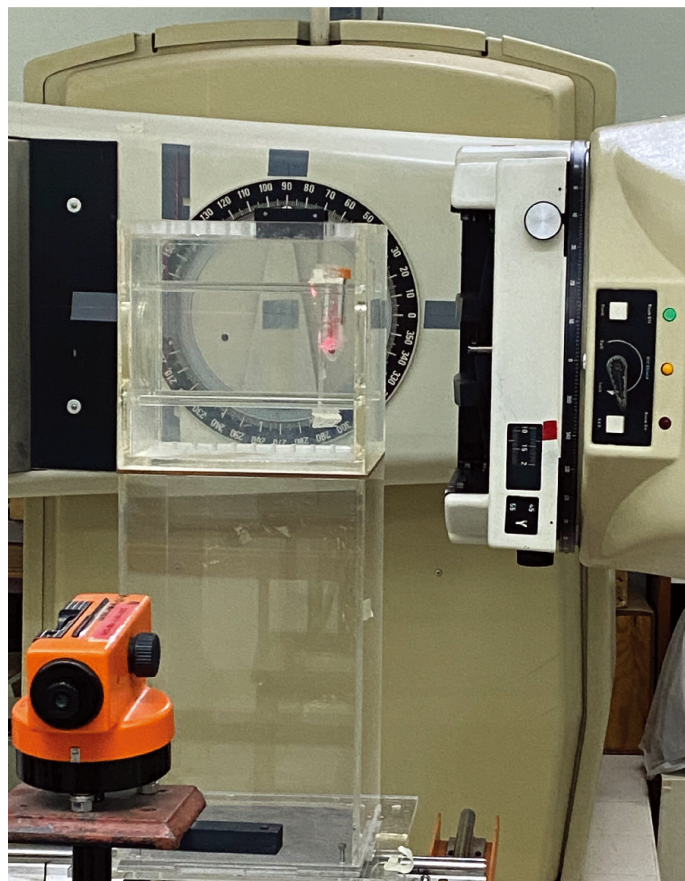
Figure 1: The setup of water phantom for the irradiation of whole blood samples by a Co-60 teletherapy machine at SSDL
