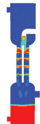
CFD simulation of an extraction column in Pakistan
