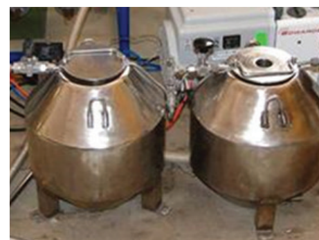
Radioactive gaseous tracer preparation system in Vietnam
