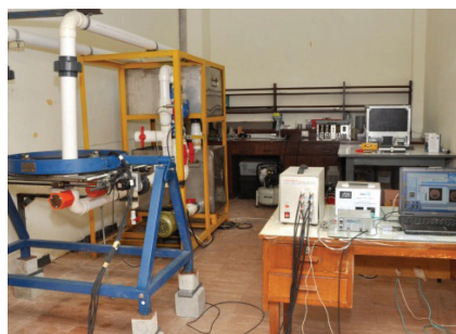
Two phase flow visualization by gamma CT system (GORBIT)
