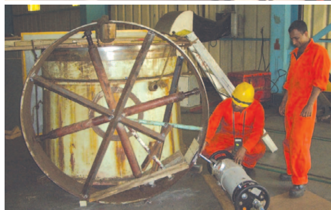
Radiographic testing of a repaired wicket gate of the Samanala Hydro Power Station of Sri Lanka
