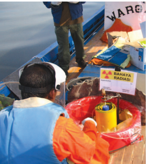
BATAN staff inject the radiotracer technetium-99m into a river entering Jakarta Bay. The survey boat follows the technetium tracer as it travels through the water.
