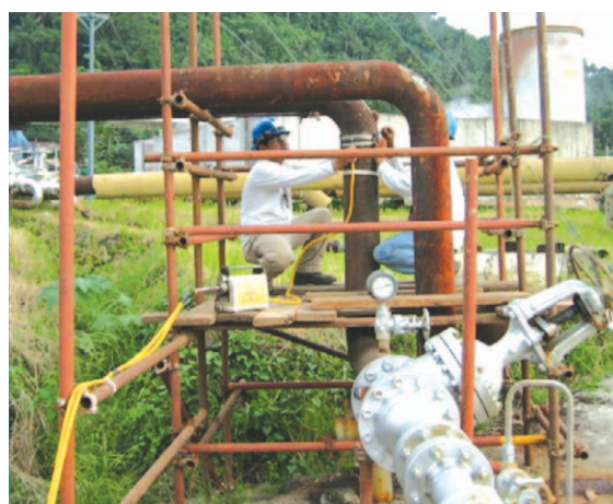
Radiographic Testing of Newly Constructed Pipeline in the Philippine Geothermal Power Plant
