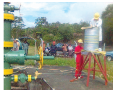
Injection of tritium tracer (370 GBq activity) at Kamojang, Indonesia for investigation of residence time and recovery of injected water
