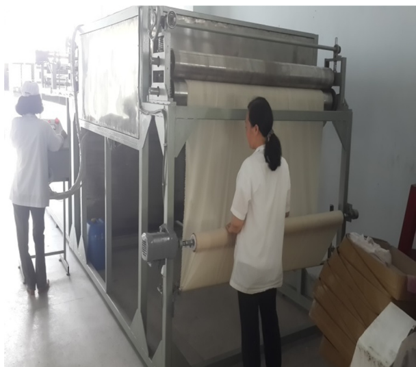
Equipment for production of Production of cotton with surface- grafted nano-silver at VINAGAMMA
