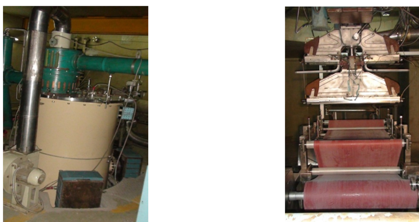
Figure 11. Upgraded EB Accelerator at BARC (Left) and Polymer Insulation Material Under the Beam Window for Irradiation in India
