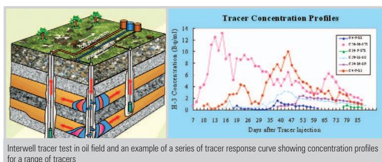
Interwell tracer test in oil field and an example of a series of tracer response curve showing concentration profiles for a range of tracers
