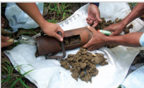
Collection of bulk core soil samples for fallout radionuclide analysis to assess soil erosion and sedimentation rates under different land uses in the Philippines
