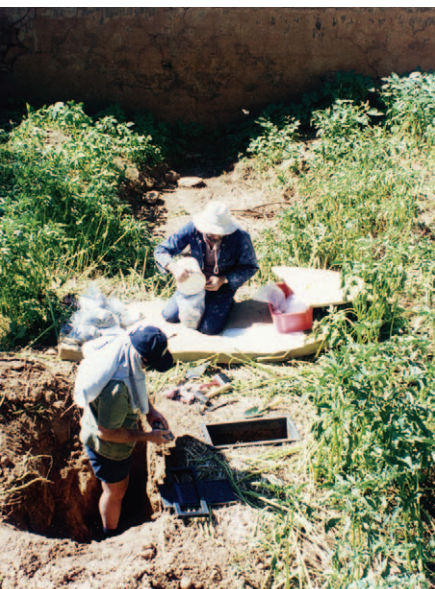
Collection of samples for the assessment of reservoir sedimentation rates in an arid environment in South East Australia using fallout radionuclide techniques
