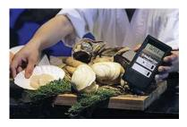
Check food for radioactive contamination with radiation meter
