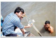
Fig. 2 Sampling of sediment with Kajak corer
